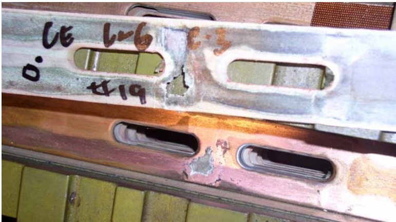
Figure 12 – Samples of Interturn Insulation with Shorted Turn Evidence
