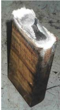
Fig. 9 – Blocking from Fig. 7 failure
